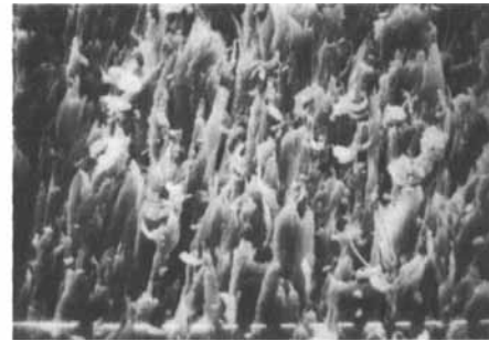
FIGURE 4d SEM photomicrograph of abraded surface of mix E. (Fibers in the longitudinal direction)
