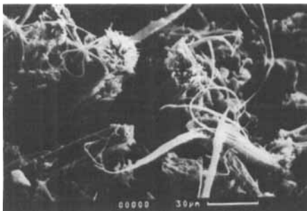
FIGURE 2e SEM photomicrograph of tear fracture surface of mix E. (Fibers in the longitudinal direction)
